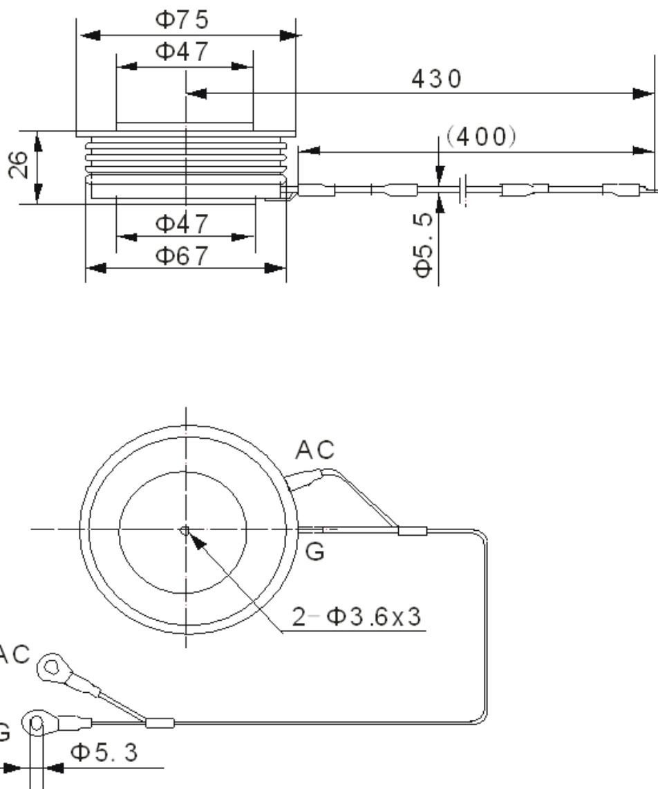
**Fig. 1** Outline drawing. All dimensions are in millimeters and represent nominal values unless stated otherwise
